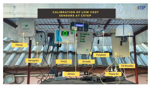
CSTEP's study noted that there are differences in the data of low-cost sensors of different make and models, and therefore, calibration models need to be make-specific.
